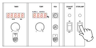
① When you are going to use the sterilamp, first close the door and turn the sterilamp switch "ON." The sterilamp bulb is turned on and the sterilamp illuminates.
