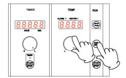
Turn the temperature setting dial to enter difference between the set temperature and the bath temperature. Turning the temperature setting dial clockwise increases setting and turning it anti-clockwise decreases it.
