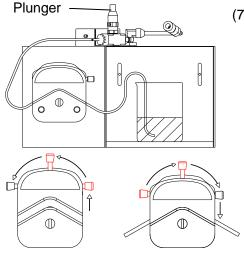
(7) Set the liquid tube as shown in the left diagram. Push the pump rod CCW to open the pump head, put the liquid sending tube in it, and then push the rod CW to have the tube stuck. Set distilled water as the specimen.
