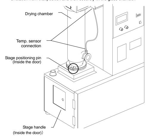
(10) Install the outlet temperature sensor into the pipe at the glass container connecting port and insert the plug into the socket on the top of the main unit.
