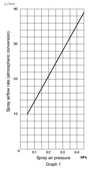
(7) The too small powder (few μ or less) among dried ones is impossible to be collected, and exhausted to the outside through the blower. If this exhausted amount of the too small powder becomes more, decrease either spray airflow rate or spray air pressure. Also, since the particle diameter becomes smaller as the density of the sample is lower, adjust the density of the sample if required.
