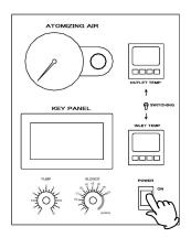
(2) Turn the power switch on the operation panel of the main unit ON.
