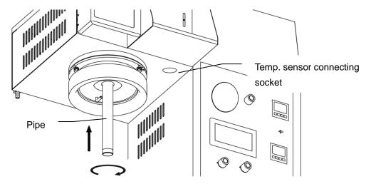
(9) Align the groove with the stage positioning pin and then install the drying chamber. Open the left side door and turn the handle while holding the drying chamber by hand to lift the stage. When the glass chamber reaches the top of the main unit, turn the handle by about half a rotation from that position and then securely fix the glass chamber.
