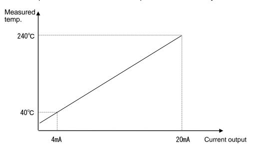
Conversion formula: Current output I (mA)=0.08 x (measured temperature T(°C)+10)
