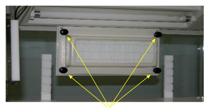
HEPA filter and housing located on the back wall of the PCR Chamber. Remove the four (4) black knobs to release filter housing.
