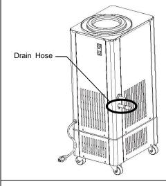
Remove the drain hose cap, and drain remaining water from the trap into a drain basin or other receptacle.
