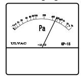
Confirm by looking at the vacuum gauge, that vacuum chamber has sufficiently decompressed. (10Pa-20Pa)
