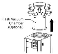
Remove the flask mounting vacuum chamber from
