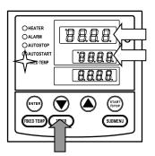
This operation is used to specify the period up to automatic stop, i.e., sets the auto stop timer during operation.
