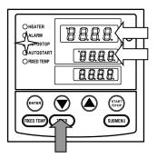
This operation is used to specify the automatic stop time in the fixed temperature operation.
