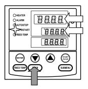
This operation is used to specify the period up to automatic start after power on.
