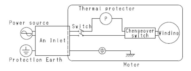
Fig. 7 Electric wiring diagram
