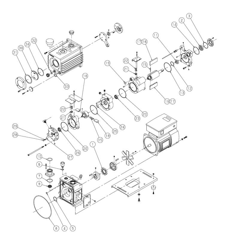
Fig. 12 Disassembly drawing of GLD-136C/201B oil sealed rotary vacuum pump
