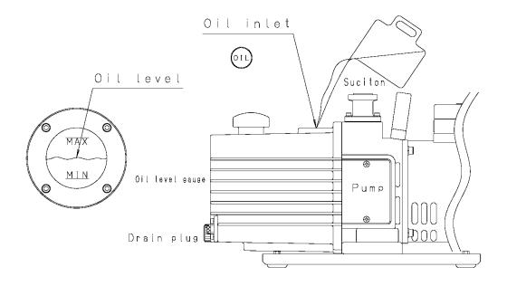
(1) Oil level shown on the oil level gauge
