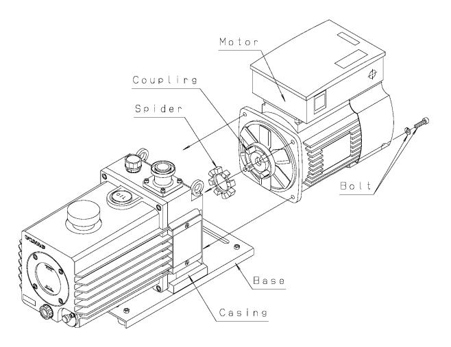
Fig. 11 Replacement of the coupling spider
