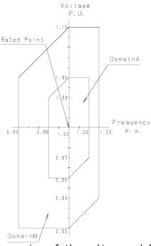
Fig. 9 Change region of the voltage and frequency
