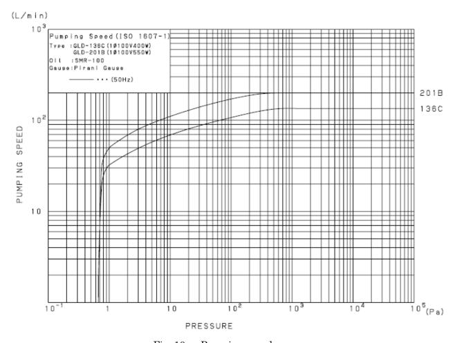
Fig. 10 Pumping speed curve
