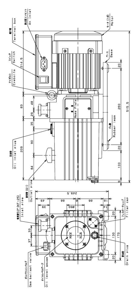
Fig. 2 Dimensional drawing of GLD-201B oil sealed rotary vacuum pump
