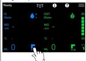
Touch the water dispense mode on the left side of the operation panel to display the window for selecting the dispense mode.
