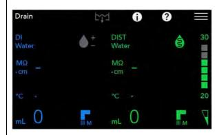
If the breaker has been turned off  $(\circ)$  for 10 minutes or more, the boiler will be drained at the same time as the home is displayed.
