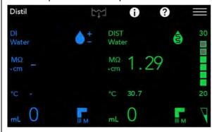
You can change the start / stop of distillation operation by touching the tank gauge. When the distillation operation is stopped, is displayed at the top of the tank gauge.
