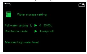
The following operations can be performed on the tank water storage amount setting screen.
