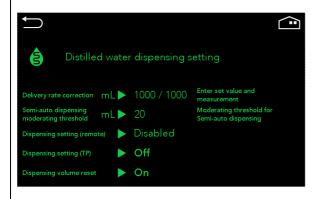
The following operations can be performed on the deionized water / distilled water dispensing setting screen.
