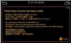
Some consumables require initial cleaning of the consumables after the integration reset. Follow the instructions on the screen and touch START at the bottom right of the screen to perform initial cleaning of consumables. Cleaning is completed when about 5 L of water is flowed, and the screen moves to the details screen of the replaced consumables.
