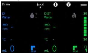
Dispenser tray drain does not work while distillation is stopped or when deionized water is sampled. You can operate it manually by touching the dispenser tray drain icon at the top of the screen. During manual drainage of the dispenser tray, "Drain" is displayed at the upper left of the screen, and the dispenser tray drain icon remains white and the following animation is displayed.
