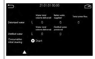
On the user maintenance screen, you can check the regular maintenance date and the usage status of the device.
