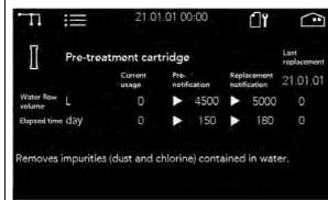
On the consumables details screen, you can check the usage status of consumables and the timing of pre-notification and replacement notification. If pre-notification or replacement notification has occurred, the name of the consumable item and the value corresponding to the notification will light orange.
