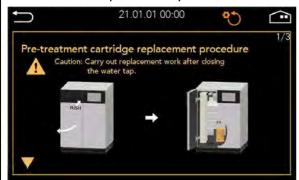
When replacing various consumables, a simple replacement procedure is displayed (the figure on the left shows the replacement procedures for the pretreatment cartridge). Touch at the bottom left of the screen to move to the next step.
