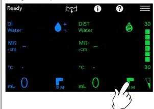
Touch the water dispense mode on the right side of the operation panel to display the window for selecting the dispense mode.
