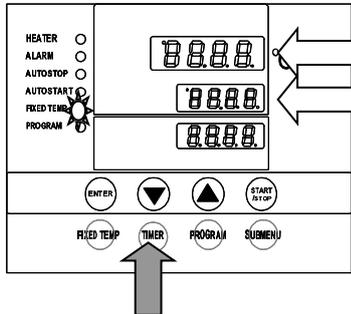
This operation is used to specify the period up to automatic stop, i.e., sets the auto stop timer during operation.
