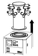
Remove the flask mounting vacuum chamber from
