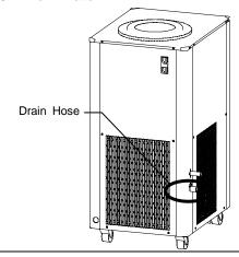
Remove the drain hose cap, and drain remaining water from the trap into a drain basin or other receptacle.
