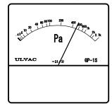
Confirm by looking at the vacuum gauge, that vacuum chamber has sufficiently decompressed. (10Pa-20Pa)
