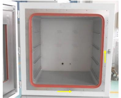
After installing the packing correctly, there is no irregularity on the surface.
