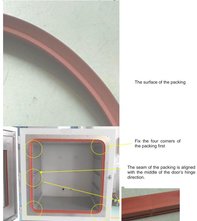
(4)While fixing the rubber with a hammer, fix the center of the four sides of the packing.
