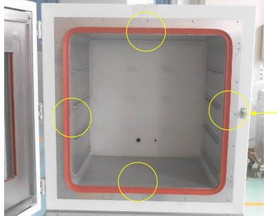
Fix the center of the four sides of the packing.
