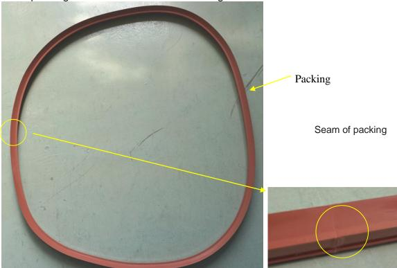
(3)Attach the packing attachment part by hammering the surface of the packing with a rubber hammer (so as not to use much force), make the lengths of the four sides of the paddle even, and set the four corners of the packing.
