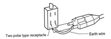
Insert the grounding adapter which is non-standard accessory into the power plug and confirm the polarity of the receptacle side, then connect it. Connect the earth wire of the grounding adapter (green) to the grounding terminal on the power facility side.
