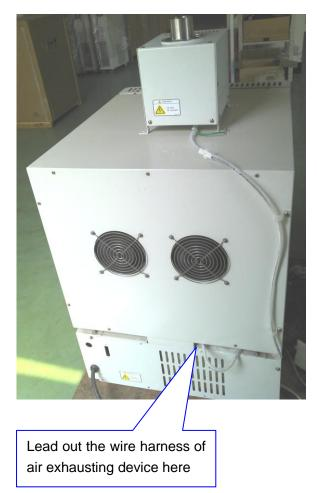
Notice: when completing assembly, if the equipment is power-on, the air exhausting device will run at once. If not use the air exhausting device, please pull out the wiring of step 4, and take the exhausting device away from the equipment.
