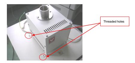
3. Fix the air exhausting device.
