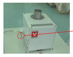
Before fixing left-rear screw, put internal tooth washer to ground between the main unit and air exhausting device, and then tighten the screw.
