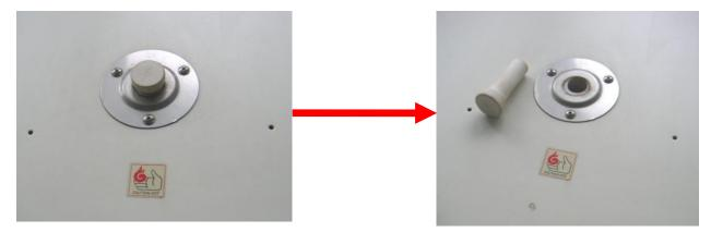
2. Put the air exhausting device on the equipment, corresponding to threaded
