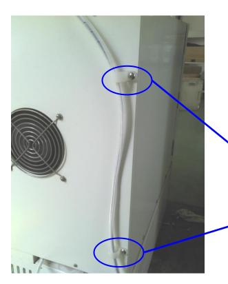
Disassemble the original screws, and use accessory 2-M4X8 big flat head screws to fix the cable clips. Do not screw tightly too much.
